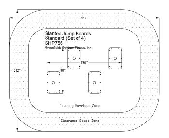
The finished surface level should be flush with the surrounding area's surface to avoid injury and provide easy access to the training area.
